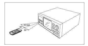
When operating the remote control, point the remote control's infrared signal transmitter at the remote control receiver (remote sensor) on the front panel of the changer. The remote control has a range of about 23 feet from the remote sensor, and within angles of up to about 30 degrees.
